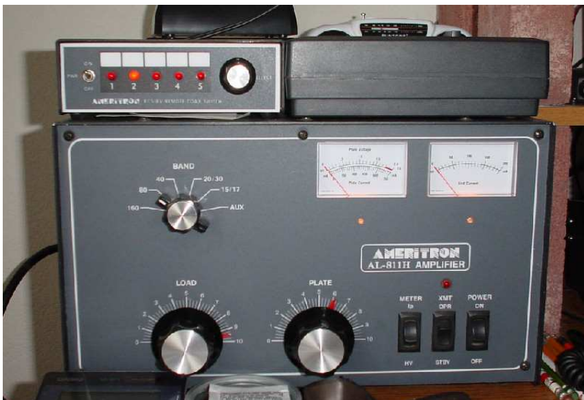
Lower left: Ameritron AL-811H 800W HF linear amplifier and Ameritron 5-position remote antenna switch controller.
